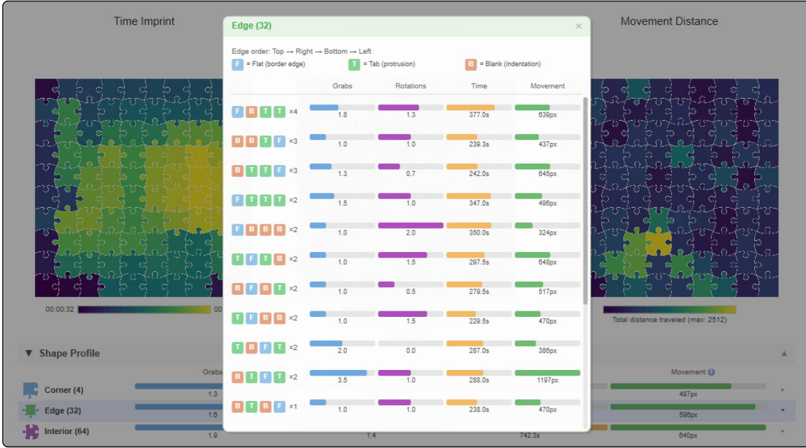
Figure 4: Second-level drill-down view of the Shape Profile component. After selecting the Edge category in the panel, this view allows pieces with similar geometric configurations to be compared within the broader edge-piece category.
